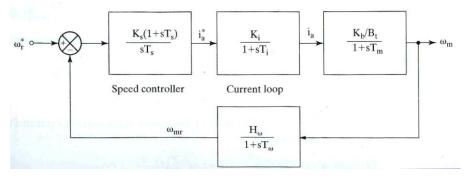
If we consider the speed feedback transfer function to be unity, we get simplified open loop transfer function of order 3. But for calculation purposes we need to reduce it to standard second order function(using pole zero cancellation method) for which the speed time constant is designed equal to Tm.i.e.  $T_s = T_m$
