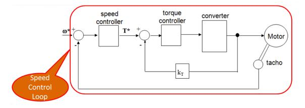
The following proceeds with deriving the transfer functions of the individual blocks of the motor and then developing analytical method to determine the controller constants.
